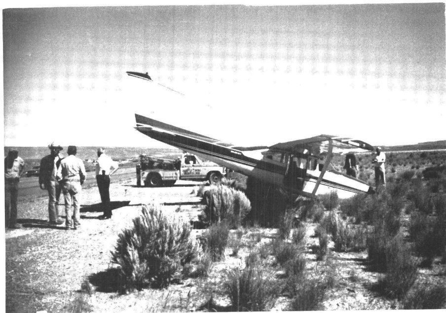
Tom Daly had a problem when the nosegear of his Turbo RG wouldn't extend at Jackpot.
