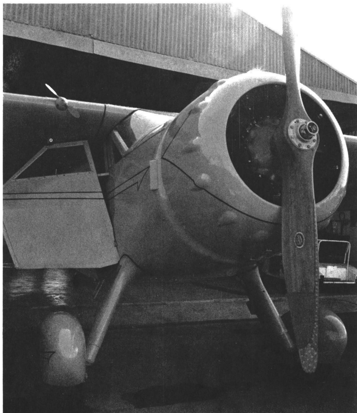
1939 Cessna Airmaster, the most efficient personal airplane of its day. Note the beany propeller of the wind-driven generator in the right wing leading edge!
