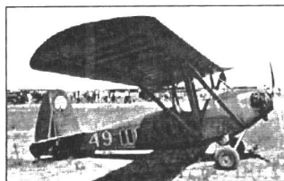
Heath Parasol, 1932. Continental A-40 engine, 40 hp. Photo courtesy of Aerofiles
