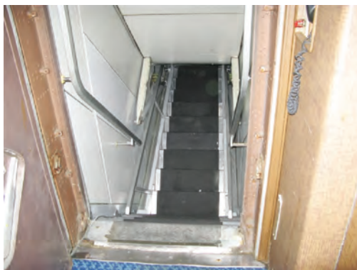
Typical retractable rear stairwell installed on B727
