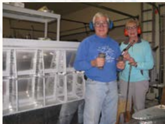
Marti and I riveting one of the RV-14A wings in our garage in Grand Junction. We built everything at home and did final assembly in our hangar.
