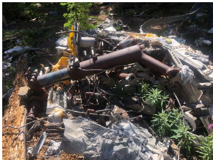
Right main landing gear attached to melted spar
