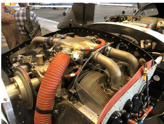
The Continental engines have routinely reached TBO with no cylinder work
