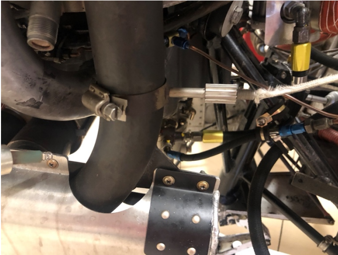
This mounted probe from a different manufacturer features cooling fins to dissipate some of the incredible heat the probe experiences.
