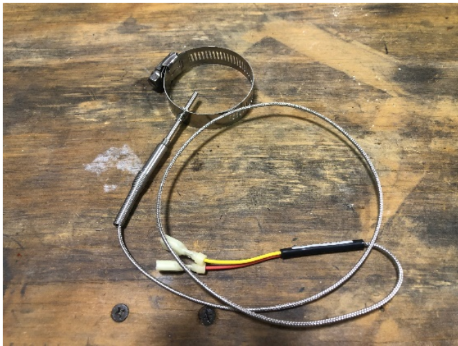
An EGT probe on the bench. The actual sensor is the small pin projecting into the circular clamp.
