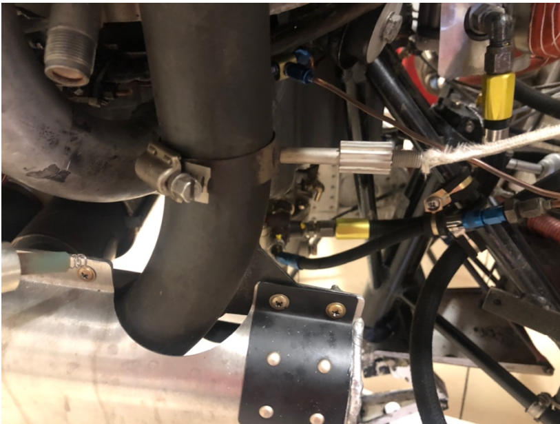
This mounted probe from a different manufacturer features cooling fins to dissipate some of the incredible heat the sensor experiences.
