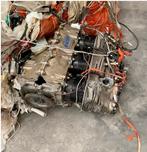
The engine and a section of parachute torn from its container
