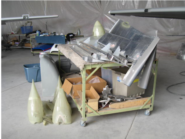
A lot of parts come off first whether it has existing paint to be stripped to bare metal or like our RV-14A, shown here, has never been painted.
