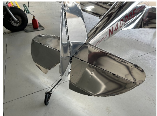
Minimizing parts count reduces cost. Both elevators are identical and interchangeable.
